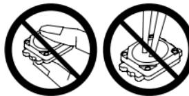
Do not touch the REGGIANI LED LUCE, in particular with sharp objects that could damage the internal connections.
